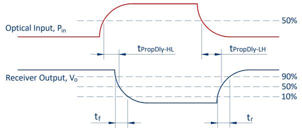
FIGURE 3 Receiver Propagation Delay and rise/fall time definitions for an inverting  $V_0$  output. Polarity of  $V_0$  is reversed for the non-inverting option.
