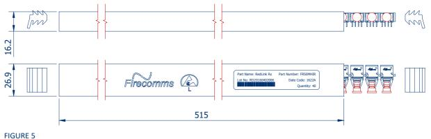
Packing tube for Firecomms Horizontal RedLink Receivers
